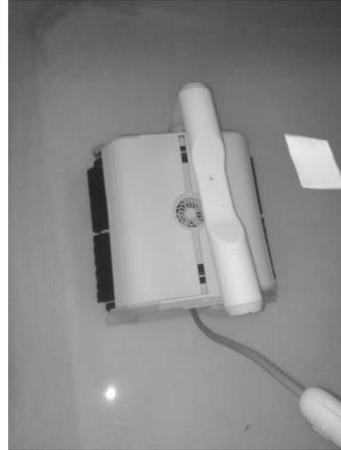
When pulling cleaner out of water, suspend the cleaner above water for about 10-15 seconds to empty the water inside.
